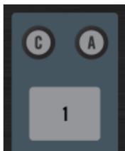
The Deck Focus buttons C and A above the left Cue/Sample Trigger section on the Z2.
