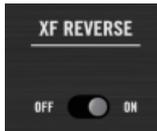
The XF REVERSE switch on the front panel.
