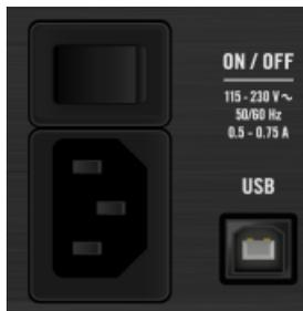
The power switch and the jack on the rear panel.
