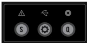
The status/mode indicators and the S (Snap), Q (Quantize), and Settings buttons below.
