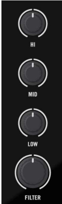
A channel's EQ (HI, MID, and LOW) and FILTER knobs on the top panel.
