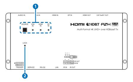
SOURCE & LEDs: Press this button to sequentially switch through the available inputs. The LED will illuminate GREEN to indicate which source is currently selected. Live, but unselected, sources will be lit RED.
