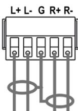
To an unbalanced stereo audio acceptor:
