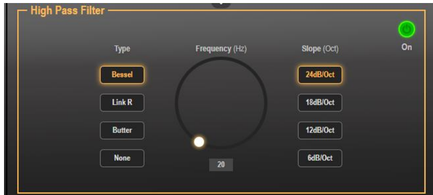
Figure 29: Processing View – HPF Module
