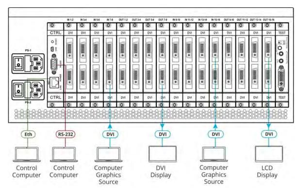
Figure 4: Connecting the VS-1616DN-EM
