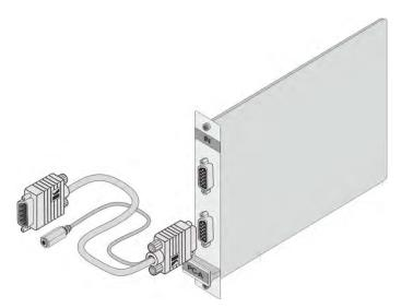
Figure 15: Accessing Audio over VGA
