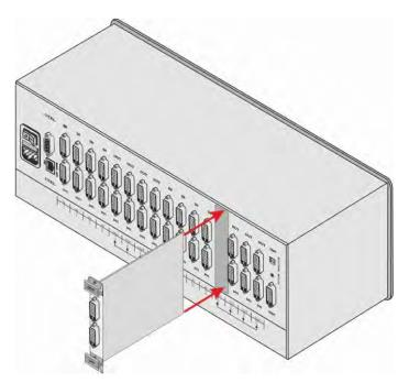
Figure 18: Inserting the Card into a Slot
