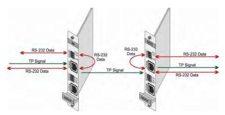
Figure 14: DGKat Card Serial Data Transmission
