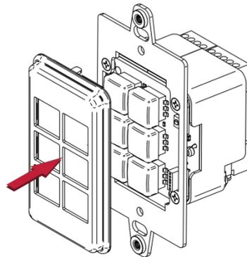
2. Use the two M3x6 screws (supplied with the kit) to attach T-1GD to the wall plate.
