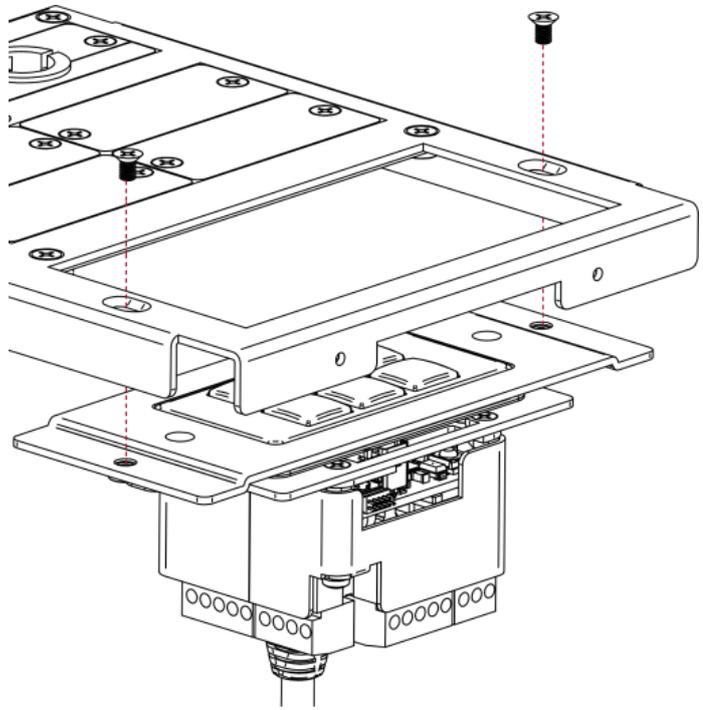
The frame can now be mounted onto the TBUS.
