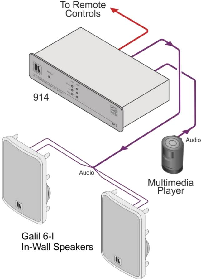
Figure 1: Galil 6-I 2-Way In-Wall Speakers in a Boardroom Setup
