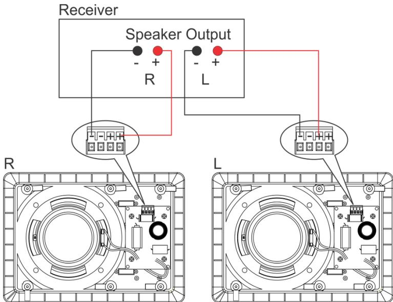
Figure 4: Galil 6-I Speakers Pinout
