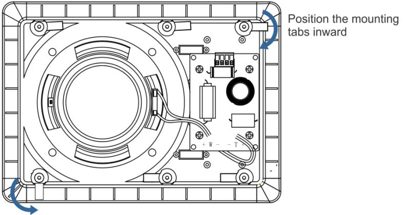
When tightening the screws, the tabs automatically turn outward
