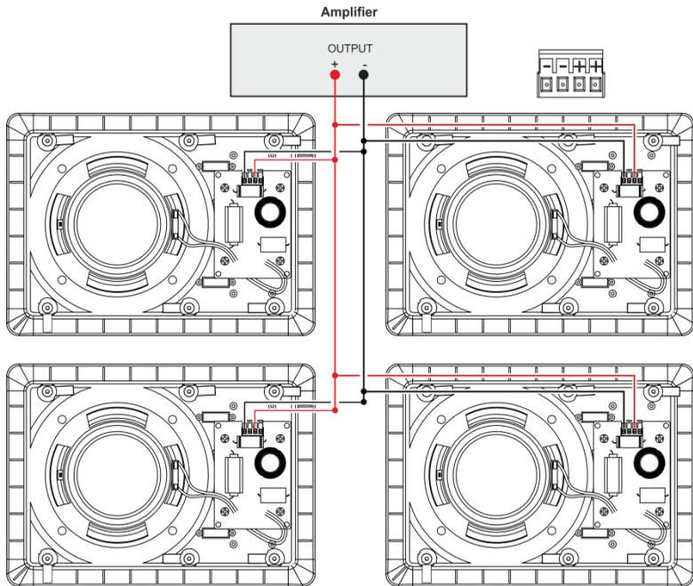
Figure 6: Square Layout Parallel Wiring
