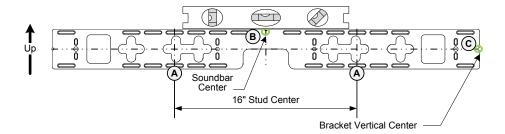
5. Attach the Soundbar to the bracket by placing the bracket's mounting bolts into the keyhole slots on the rear of the soundbar and dropping the Soundbar into place.
