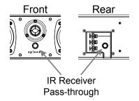
To maintain accurate IR reception, a spacer has been included to allow for the front edge of the IR receiver to be flush with the back of the grille cloth. This will ensure that IR reception is at its maximum level.
