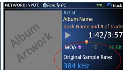
Ethernet, Wi-Fi, USB-A, and SD Card inputs are all MQA capable. *SPDIF inputs of the DMS-500-550/600 are not capable of MQA playback.* However, the DMS-550/600 can play an MQA stream from the SPDIF inputs at better than CD quality standard FLAC.
