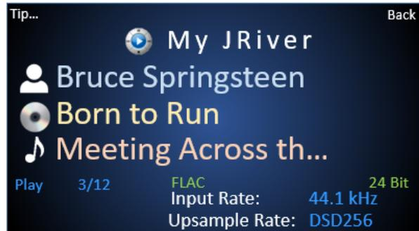
To change the DMS-500/550/600 front panel display from the default display to high contrast or large font/icon based displays, simple press this "color wheel" icon at the iOS or Android app.
