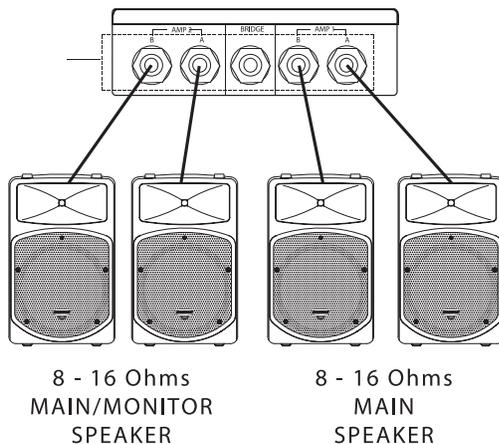
When the POWER AMPS are in BRIDGE use a speakers with a 8 – 16 ohm impedance rating.
