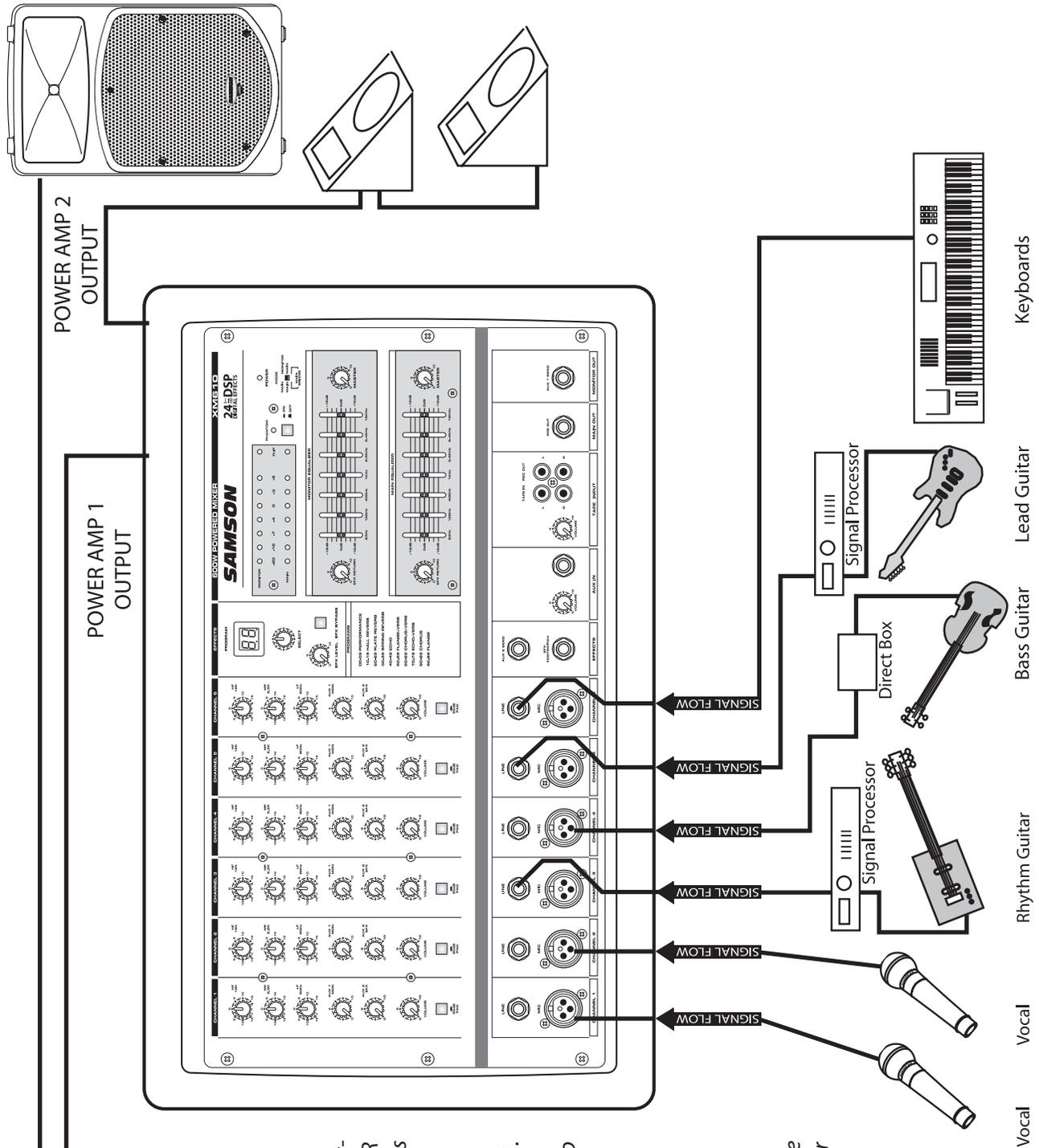
This system shows the XM610 power amp operating in MAIN/MONITOR mode, with two speakers connected to POWER AMP 2 and two monitor speakers connected to POWER AMP 1. For inputs, two microphones are connected to channel 1 and 2's low-impedance inputs, and the output of the Bass Direct Box is also connected to the Low-Impedance input on channel 4. The Keyboards, as well as the Lead and Rhythm Guitar signal processors' outputs, are connected to the XM610's line inputs.
