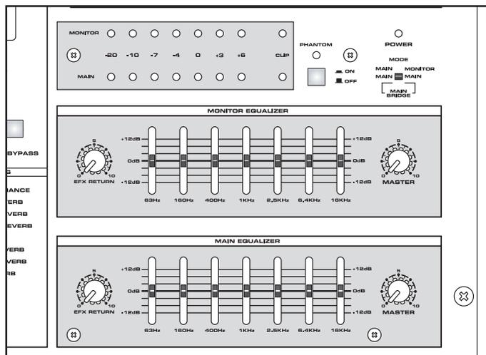
3. Use the graphic equalizer and MASTER controls of the MAIN/MONITOR sections to adjust the overall volume and tone.
