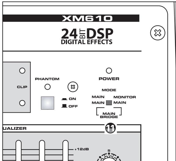
**CAUTION!** Only change the power amp mode switch when the XM610's power is **SWITCHED OFF!**
