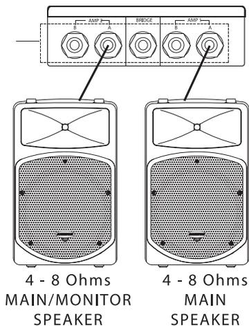
When connecting two speakers to POWER AMP 1 and two speaker to POWER AMP 2, use speakers with a 8 – 16 ohm impedance rating.
