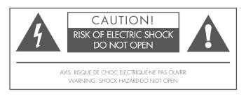
This lightning flash with arrowhead symbol within an equilateral triangle is intended to alert the user to the presence of non-insulated "dangerous voltage" within the product's enclosure that may be of sufficient magnitude to constitute a risk of electric shock.
