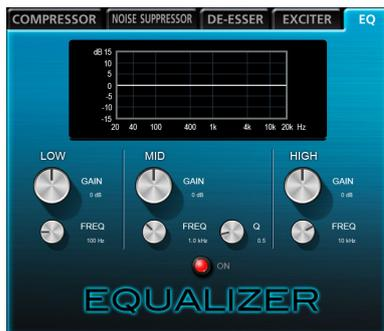
The frequency response is shown even when the equalizer is off. The equalizer has a high-shelf HIGH band, a low-shelf LOW band and a peaking (bell-shaped) MID band.
