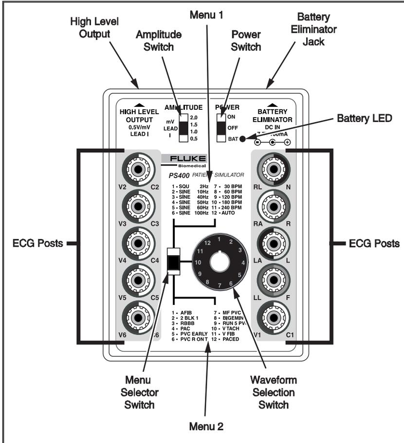
Figure 1. PS400 Controls and Indicators
