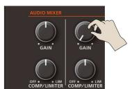
4. While producing the sound that is actually going to be input, slowly turn the [MIC 1] or [MIC 2] knob clockwise to adjust the input gain.
