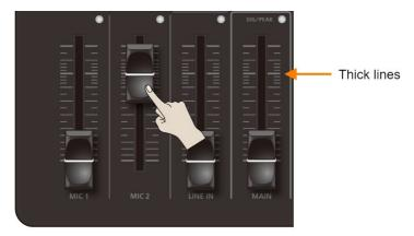
2. Move the [MAIN] fader to a position near the thick lines on the level scale.
