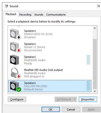
3. On the Playback tab, select "Speakers (TASCAM TM-250U)" and open the Properties window.
