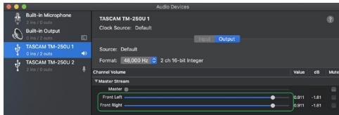
The slider opened from the speaker icon in the menu bar can also be used to adjust the overall monitoring volume of direct monitoring and Mac playback signals.
