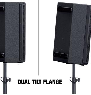
The speakers have a stand flange with a 0° angle socket (rear position) and a socket with a 5° tilt angle (front position). Examples of use: Use the socket with the 0° angle for standing audiences and the socket with the 5° tilt angle for seated audiences.
