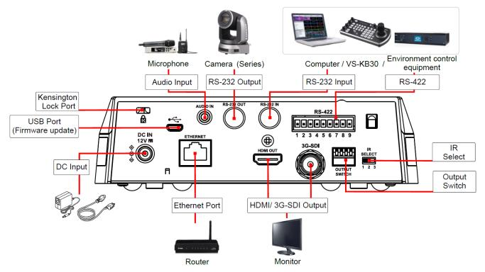
3.3.1 RS-232 connection (at most 7 Lumens cameras can be connected)
