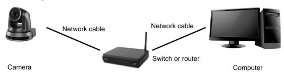
To connect directly through network cable, the IP address of the computer should be changed so that it is on the same network segment as the camera E.g.: The factory-preset default IP address of the camera is 192.168.100.150. The computer IP address must be set with the same network segment, such as 192.168.100.101, so that the computer can be connected correctly with the camera
