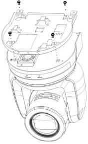
3. Lock the metal plate B on ceiling mounted hanger
