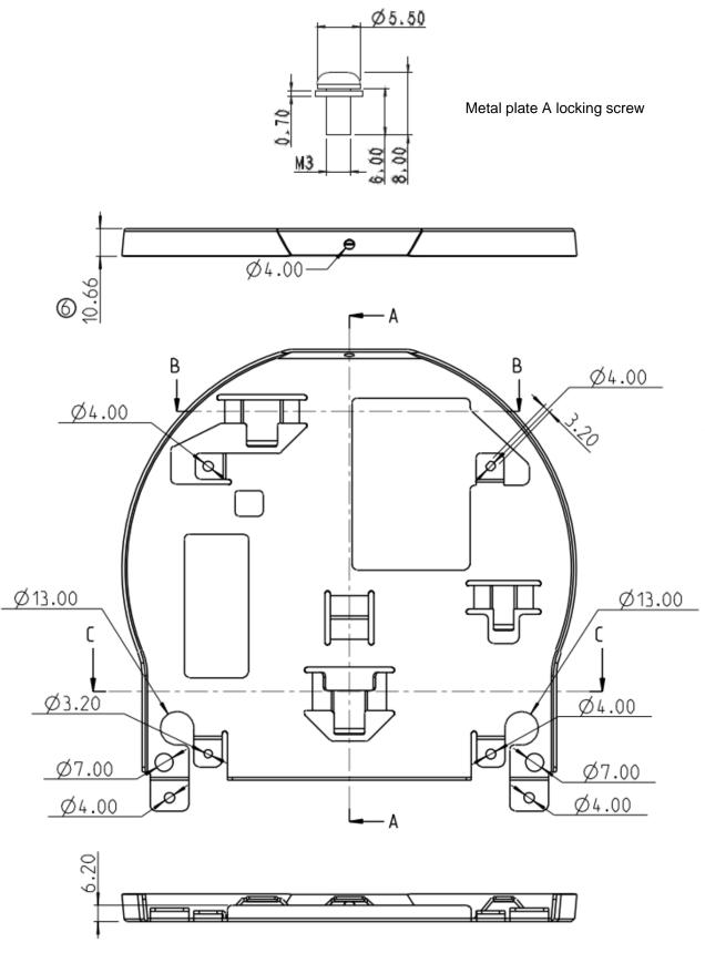
Metal plate A - machine side
