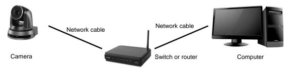
2. To connect directly through network cable, the IP address of the computer should be changed so that it is on the same network segment as the camera
