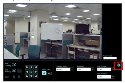
2. Use PTZ function to adjust to the screen to be partitioned, and then click to save. The partition icon below will be changed to the saved position
