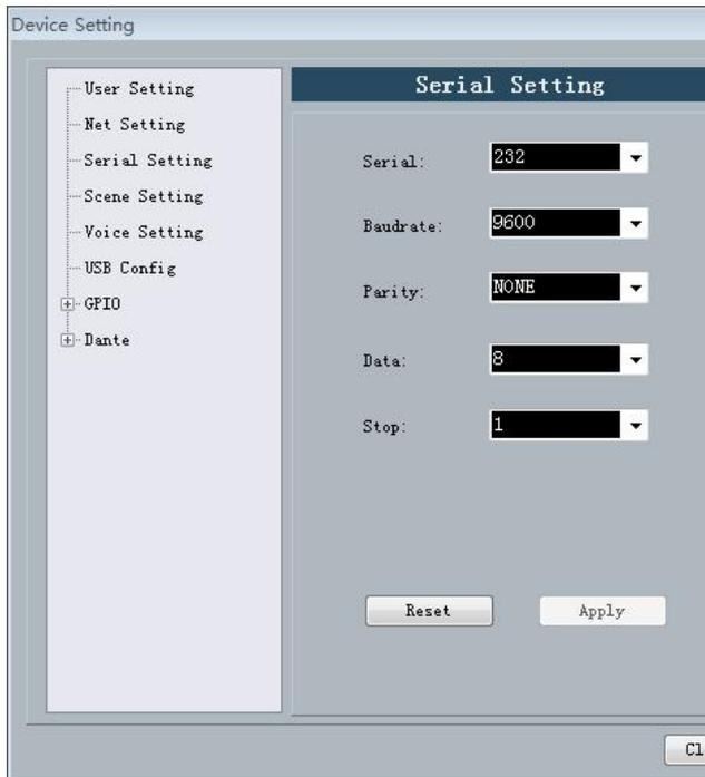
To view and modify the current equipment serial port information, set up and then click the "apply" button to modify the current equipment serial port information; If you want to return to the default, just click "reset" button, Settings cannot be empty.
