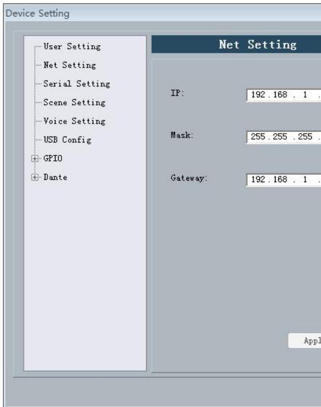
To view and modify the equipment of network address information, in the position of the corresponding input IP address, subnet mask, gateway, click apply button modification is completed.
