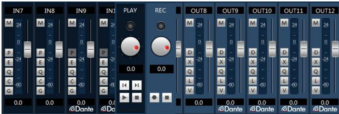
Select the Dante channel in the input part, open the input control, and in the "select device/channel" drop-down list, you can see the list of connected Dante devices and channels in the current network. Select the channel number under the corresponding device to complete the Dante access of the current channel, and the output channel of the corresponding device will become the input signal source of the current device through the Dante module.
