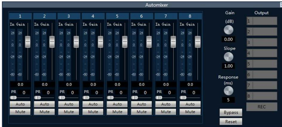
**Each channel of an automatic mixer has an input, gain level meter, and an automatic gain, channel fader , priority, and channel mute.**
