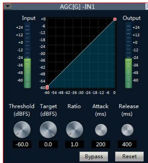
**Threshold:** When the signal level is below the threshold, the input / output ratio is 1: 1. When the signal level is above the threshold, input / output = ratio. Set this threshold level slightly above the noise ratio of your input signal.
