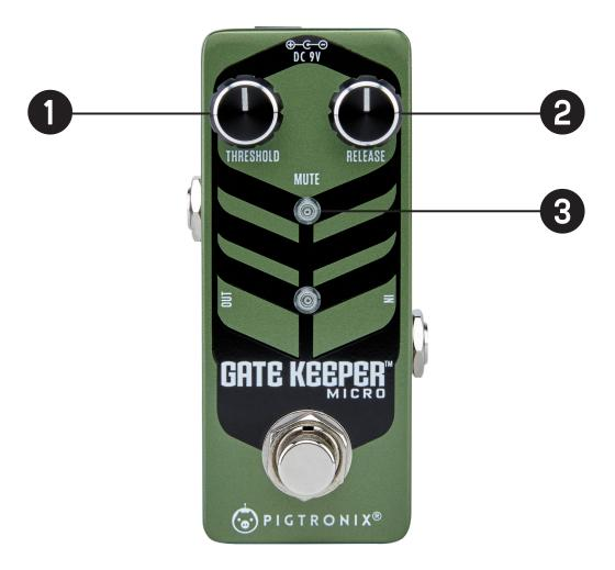
**Threshold** is the most important control on the Gatekeeper pedal. This knob controls how much signal is needed in order to open the gate. The hotter the signal you put into the Gatekeeper, the lower the Threshold knob should be set.
