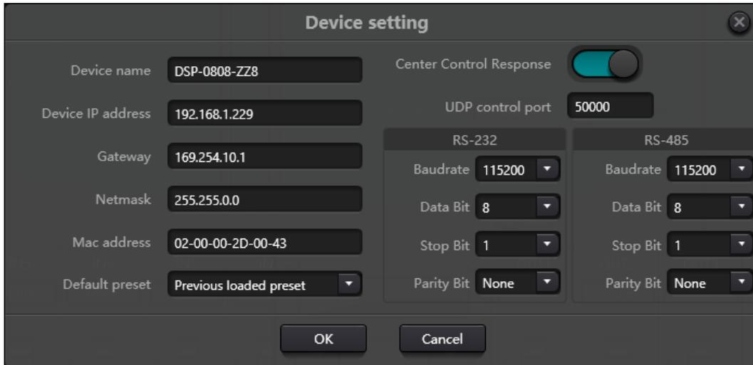
Information like device name, network address and SERBAUD can be set on device setting. The maximum length of the device name is 16 characters or 5 Chinese characters.
