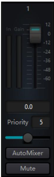
**Auto Mix:** Each channel has an automix on/off button which must be turned on for channels need to participate in automix. It may also be closed, and then the channel will not participate in automix.
