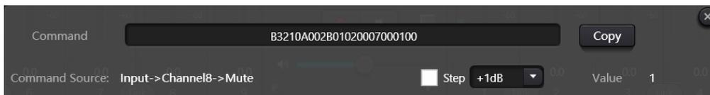
Open central control command window and click parameters to be controlled on interface, then the window will display current command immediately. Copy the command and then use UDP or RS232 to send the command to devices.
