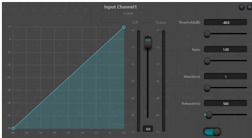
**Threshold:** When the signal level is higher than the threshold, the compressor/limiter begins to reduce the gain. Any signal that exceeds the threshold is regarded as overshoot signal, and its level will be reduced in normal cases. To a greater extent the signal exceeds the threshold, more level is attenuated.
