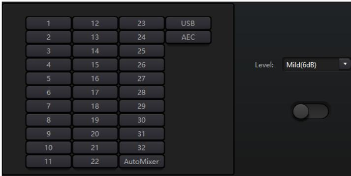
Suppression level: There are totally three levels including Mild(6dB), Medium(10dB) and Aggressive(15dB) for selection. dB here refers to the decibel of suppression noise reduction. The bigger the value, the more harm on voice generated, which is inevitable.
