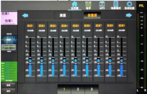
Effect volume source Displays the status of the input channel sent to the current effect
