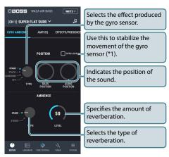
You can automatically position the sound using the gyro sensor built into the WAZA-AIR BASS, and adjust the ambience sound effect.
