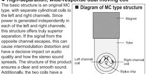
reverse-V shape which reduces effective moving mass as seen from the stylus tip, limiting unnecessary movement of the coil and further eliminating
