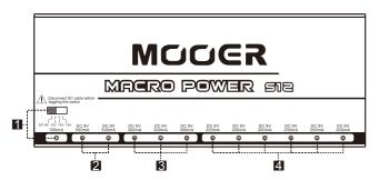
1 x 300mA DC output with selectable voltage switch. 9V, 12V, 15V or 18V
