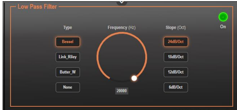
Figure 36: Processing View – Processing Output LPF
