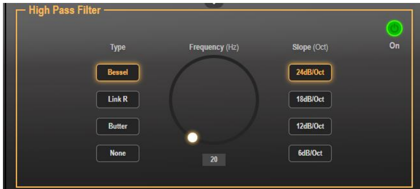
Figure 26: Processing View – HPF Module
