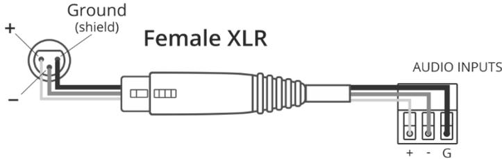
Figure 4: Connecting a Balanced XLR Input
