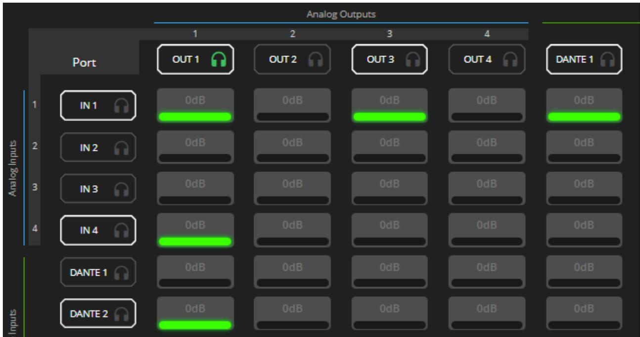
Figure 20: Matrix Page – Multiple Input-Output Cross-Point
