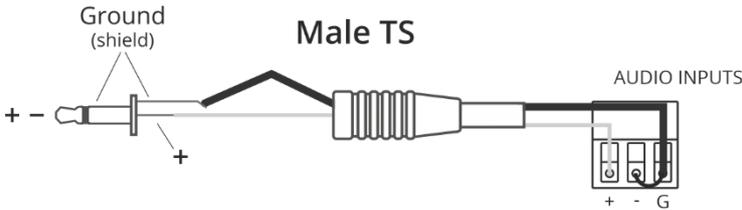
Figure 7: Connecting an Unbalanced 6.5mm Phone Jack
