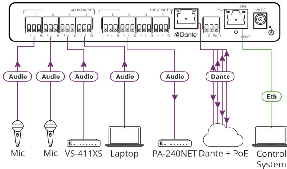
Figure 3: Connecting to the FC-404NETxl Rear Panel
