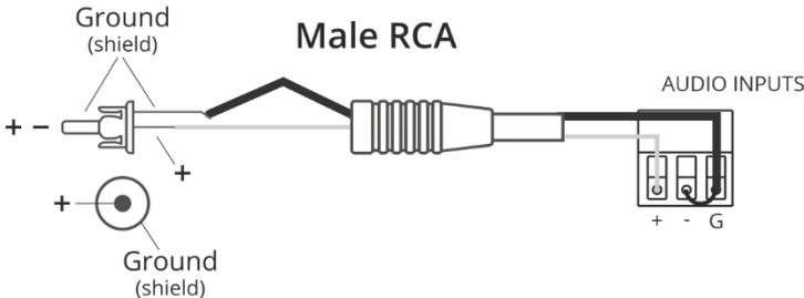
Figure 6: Connecting an Unbalanced RCA Input
