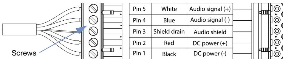
Figure 28: Pin Destinations for Phoenix 5-Pin Female Cable Mount Connector
