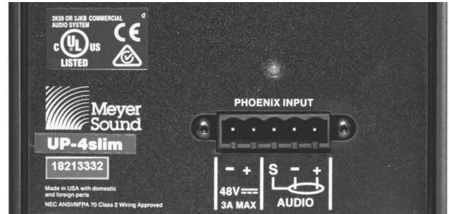
Figure 7: UP-4slim Rear Panel with Phoenix 5-pin Male Connector
