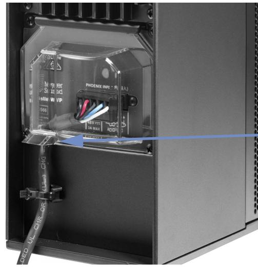
Vertical orientation: the Phoenix connector will be to the right and the cables will exit from the bottom left of the rain hood.
