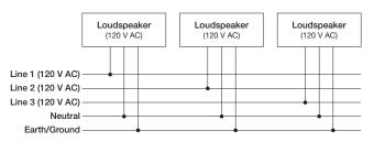
Figure 1: 120 V AC, 3-Phase Wye System (Single Line to Loudspeakers)
