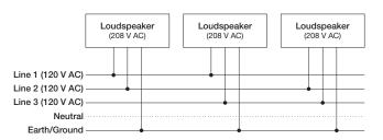
Figure 2: 120 V AC, 3-Phase Wye System (Two Lines to Loudspeakers)
