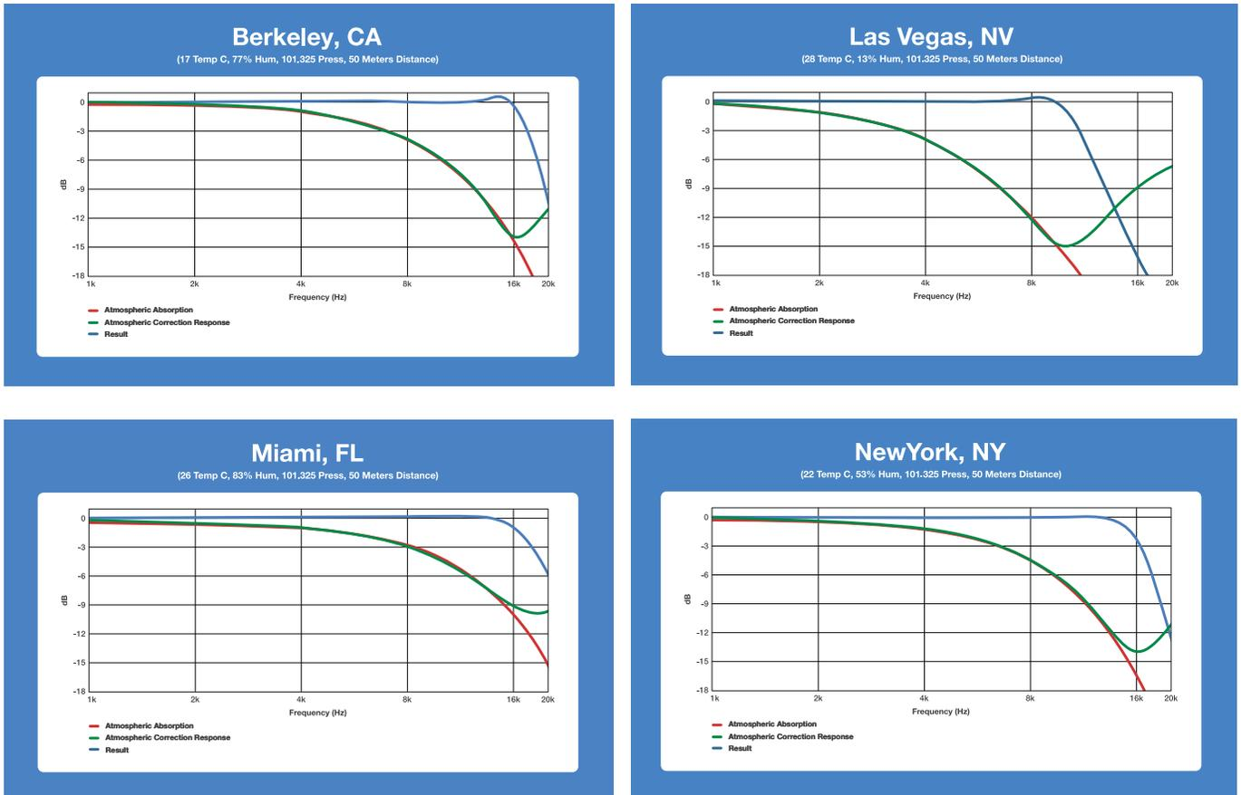
Figure 40: Atmospheric Correction Results for Four Different Scenarios.
