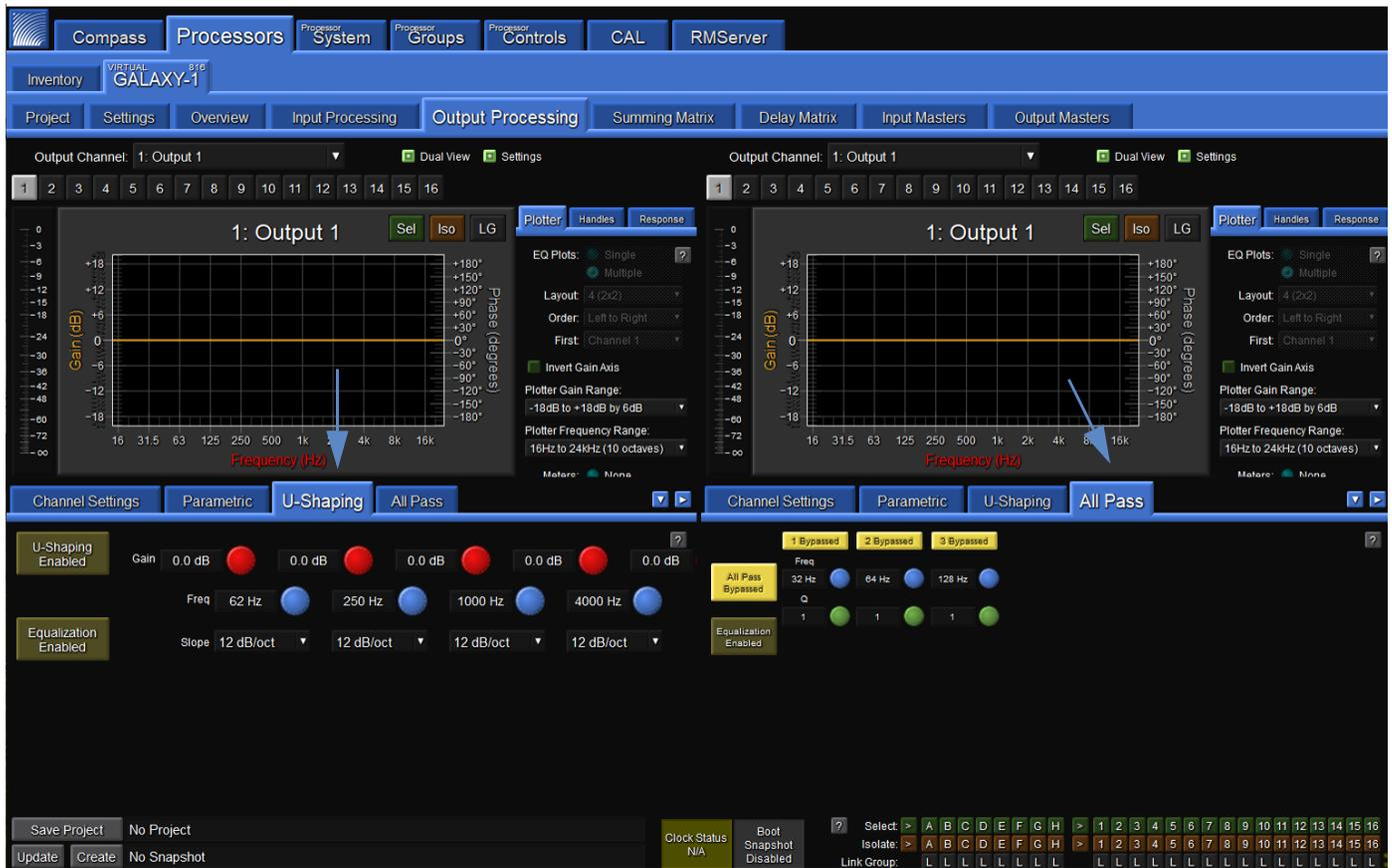
Figure 20: Processor > Output Processing > U-Shaping and All Pass tabs
