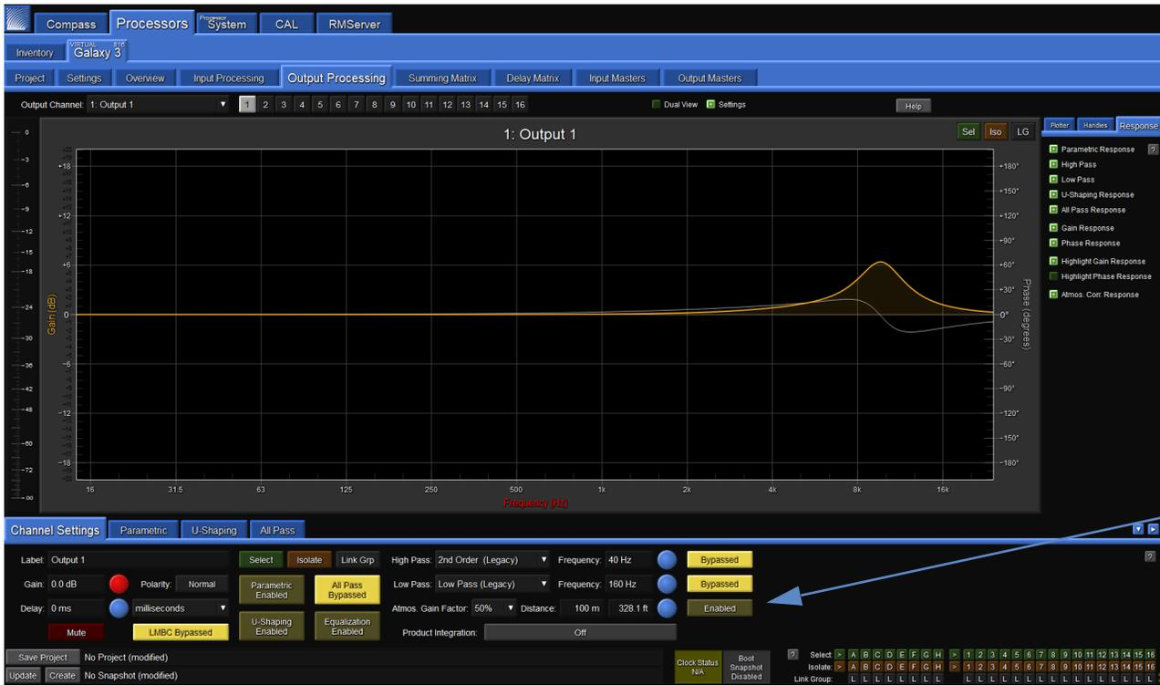
Figure 43: Atmospheric Correction Enabled and Displayed
