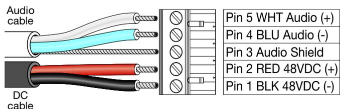
Separate Cables for DC Power and Balanced Audio
