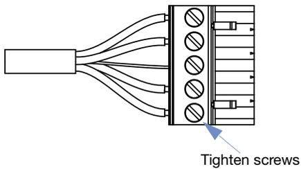
**CAUTION:** Screws should not be inserted into the Phoenix connector while the connector rests in a mating plug. Doing so will damage the contacts. During assembly, the Phoenix connector should only be held in place externally.
