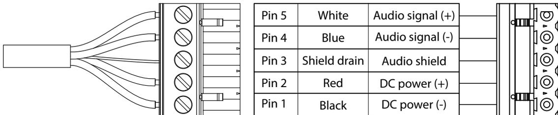
*Pin Destinations for Phoenix 5-Pin Female Cable Mount Connector*
