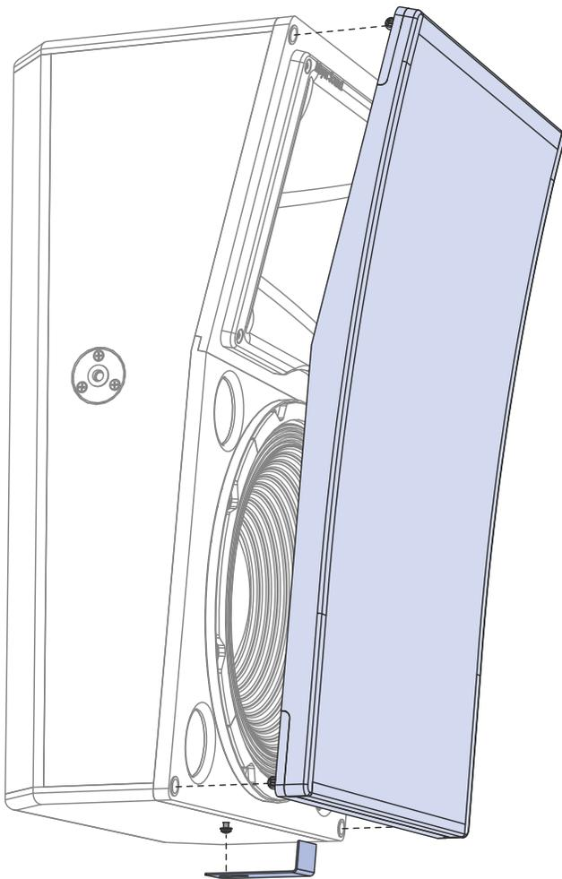
2. Re-tighten the pan head screw without the L-bracket installed.
