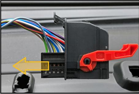
7. Remove the connector from the housing.
