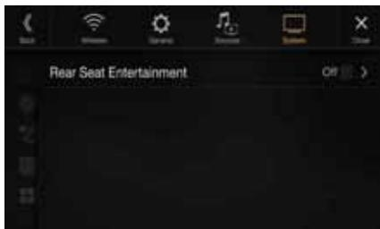
When a Rear monitor equipped with HDMI input is connected to this unit, change this setting to "On." You can output images to the Rear monitor. For details, see "Rear Seat Entertainment Function" (page 18).
