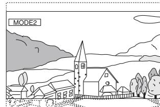
In Mode 2 (Cinema), the monitor displays a normal picture by stretching out the picture horizontally and vertically. This mode is good for displaying a cinema type picture at the 16:9 ratio.
