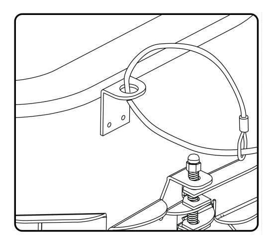
4. Place the loudspeaker in the mounting hole. Tighten the screw on each side of the loudspeaker until each mounting arm fully expands to the secure the loudspeaker. Do not over-tighten the screws.
