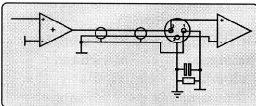
To connect an input to an unbalanced source, it is possible to connect pins 1 and 3 in the XLR plug at the amplifier end of the cable. However, a better method is to connect pin 3 to the shield at the source end of the cable, as this usually results in better hum and noise rejection. Balanced input connections are recommended whenever possible
