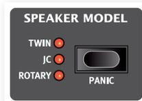
JC and Twin emulates two different kinds of amplifier and speaker cabinets. The amount of overdrive is controlled by the Drive Amount controls to the upper right on the panel.
