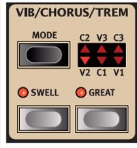
Three different types of choruses (C1 - C3) and three different types of vibratos (V1 - V3) are available. Select one of these types by pressing the Mode button. The effect can be activated/deactivated for both manuals individually by pressing the Vibrato/Chorus button for the swell and great manuals.
