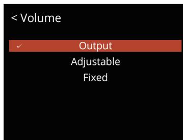
When set to ADJUSTABLE, the D9 Volume control is used to adjust the level of the analogue output. This is required when connecting directly to a power amplifier. The default setting on the D9 is ADJUSTABLE.
