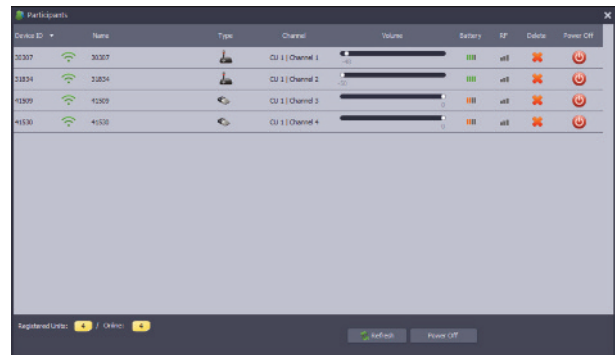
Participants - four microphones are allocated to all audio channels of one control unit
