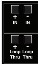
To wire Control 40 Series loudspeakers simply connect the positive wire to the “+” pin and connect the negative wire to the “-” pin. The “IN” pins are paralleled to the “LOOP THRU” pins (+ and - respectively) inside the loudspeaker. The “Loop Thru” pins allow a parallel connection to an additional loudspeaker.
