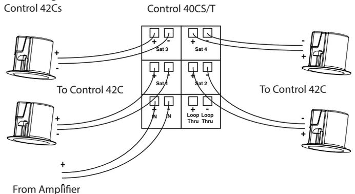
Use only either two or four satellite loudspeakers as described in the recommended configurations. Do not use one or three satellite speakers, or it could result in uneven sound levels and / or damage to your sound system.
