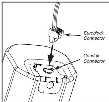
4. Loosen the conduit connector on the input terminal cover and insert the wired euroblock connector through the conduit connector opening. Connect the euroblock to the matching receptacle.
