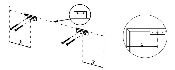
**Step 11.** Position the fixed frame screen onto the top wall brackets as shown below and push down at the center of the top of the frame to secure.
