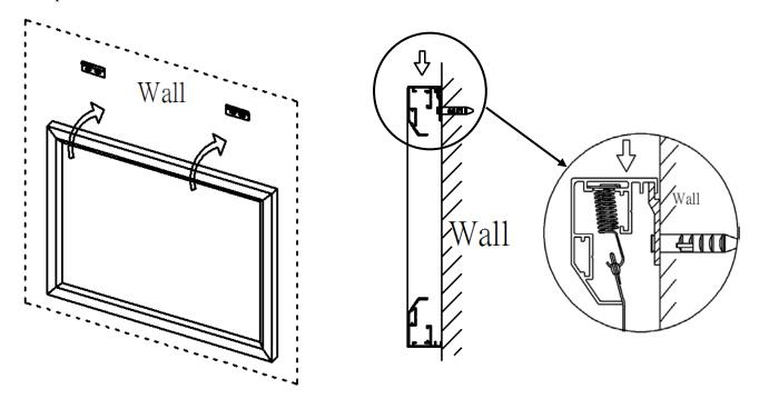
**Step 12.**With the frame slightly tilted outward; connect the bottom brackets onto the bottom groove of the frame. Slowly return the screen to a normal upright position. Once the screen is flush to the wall, secure the brackets to the wall with a screw. If not installing into a structural wood stud, mark the sites where the hollow wall anchors will be placed using the same instructions above. With the wood anchor installed, repeat the process and fasten the brackets with the M5x50 wood screws.
