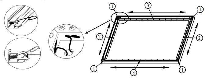
**Step 9.** Insert the Center Support Bar into the upper top groove on the back of the frame (not the one where the spring inserts) with the bottom end near the approximate center point of the frame. Rotate it in at an angle so that both ends of the bar are in alignment with the groove. (See illustrations below for details)
