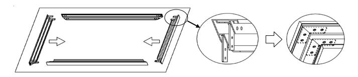
**Step 6.** Secure the elbow joints by fastening them with 4 M4x6 screws (4 at each corner). Do no tighten completely until all frame pieces are assembled correctly.
