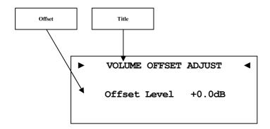
To offset differences between input devices, you can adjust the volume level for each channel in range from -9dB to +9dB.
