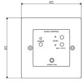
Dimensions: 85 x 85 x 35mm (h x w x d) Weight: 75g Input sensitivity stereo line: 500mV
