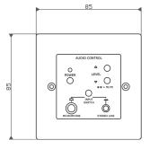
Dimensions: 85 x 85 x 28mm (h x w x d) Weight: 90g Input sensitivity stereo line: 500mV Input sensitivity microphone: 7mV
