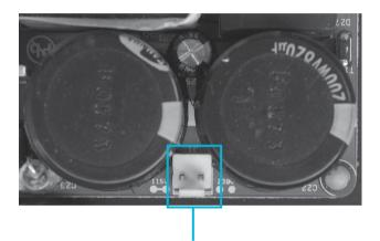
110 VAC operation: it is possible to operate the unit at 110 (115) VAC.
