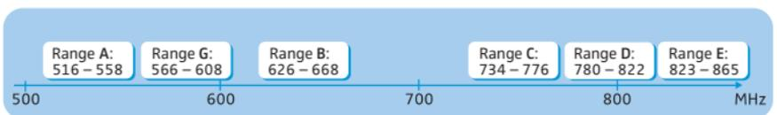
Each frequency range (A–E, G) offers 21 frequency banks with up to 12 channels each:
