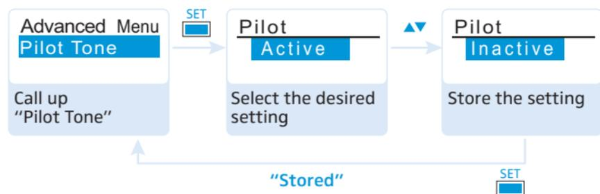
The plug-on transmitter adds an inaudible pilot tone to the audio signal. The receiver detects and evaluates the pilot tone, and is thus able to identify the signal of the matching transmitter and mute all others. The pilot tone supports the receiver’s squelch function.
