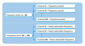
Each of the channels in the frequency banks "1" to "20" has been factory-preset to a fixed transmission frequency (frequency preset). The factory-preset frequencies within one frequency bank are intermodulation-free. These frequencies cannot be changed.
