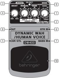
3 The **MANUAL** control determines the wah effects' lowest frequency. In HUMAN VOICE mode, it selects the second vowel. In TEMPO mode, this control has no function.
