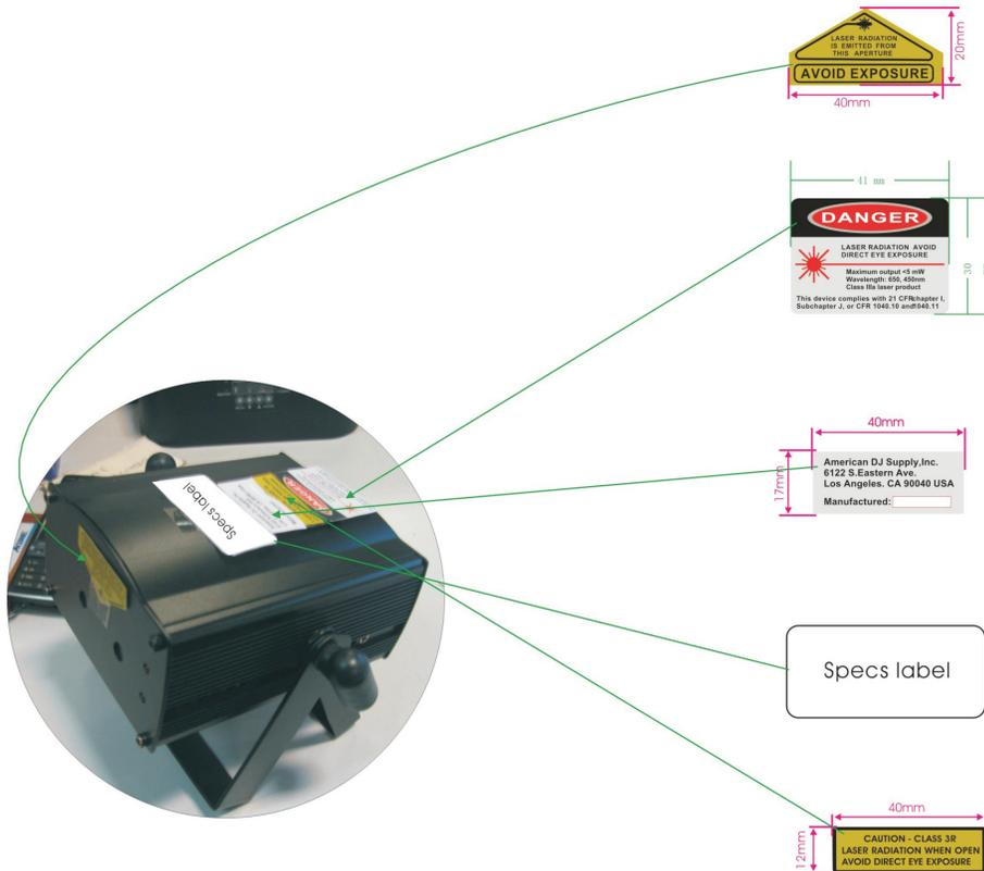
**CAUTION IMPORTANT!** When installing this projector, make sure that it is mounted in a manner that prevents the audience from looking directly into the beam, and the beam from striking the audience.
