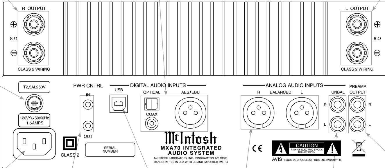
PWR CNTRL (Power Control) IN receives a turn On/Off signal from a McIntosh Component; PWR CNTRL OUT sends a turn On/Off signal to an other McIntosh Component
