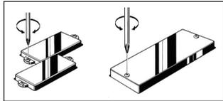
\*Instruments that have adjustable pole pieces can be adjusted to balance the output of each string.
