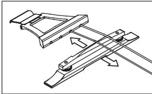
You need to loosen the strings to make adjustments, but this may cause the bridge to move too much. If this occurs, adjustment will be easier if you aim for a scale length of 770mm/30.3" between the nut (0 fret) and saddle of the first string. Once the adjustment is made, change strings one at a time to minimize saddle movement.
