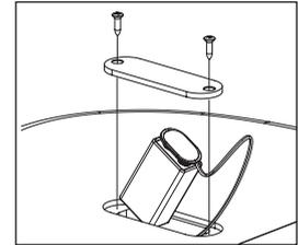
Inserting a plug into the output jack activates the power supply. Unplug the instrument cable when bass is not in use in order to reduce drain on the battery.
