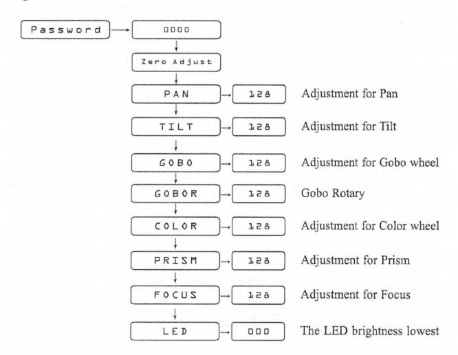
Press the <UP> <DOWN> button repeatedly until you reach the desired adjustment, Press the <ENTER> button to confirmed. Confirmed. It will auto exit after 10 seconds. Press the <UP> <DOWN> button repeatedly until you reach the desired adjustment, Press the <ENTER> button to confirmed. Confirmed. It will auto exit after 10 seconds.
